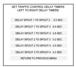
Even if your equipment only has 2 or 3 fill spouts timers for a maximum of 4 spouts are shown. Leave timer values at 0.0 for unused spouts. Delay timer for spout 1 to spout 2 amount of time from the instant the bag chair is actuated for spout #1 to the instant the bag from spout #1 enters the area of interference for spout #2.
