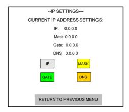
Select each of the 4 boxes and enter a valid address. If, for example the address being entered is 255.0.255.255, then enter the string as follows:
