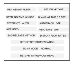
Description of the first 7 variables on this screen are described in sections 5.2, above. Items unique to the Net Weigh controller include Bag Release Method and Dump Mode.
