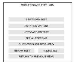
The Sawtooth test is conducted at Thompson Scale Company and requires connection of an oscilloscope. We use this as one of our final tests prior to releasing a new 5511/6611 for shipment. It is not intended for field use.
