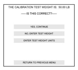
If the test weight value is incorrect, select "No, Enter Test Weight", and a screen will appear for entry of this value. A button is also available for changing the calibration weight units.
