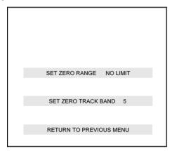
This routine can automatically zero any deviation from the current operating zero, up to 2%, 5%, 10%, or unlimited % of the test weight size. See Calibration Chapter 3 for information on selecting the proper test weight for your scale. Each time the zero is updated, an "AZ" symbol appears on the Run screen, just to the right of the weight display.
