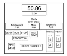
The filler will only operate when in this screen. To start the fill process, press the "Run" button.
