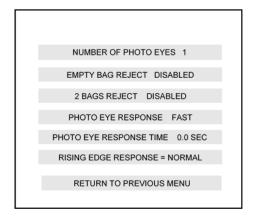
However, this doesn't always fit every application, and some require either a weight terminating photo-eye at the exit of the conveyor, or a combination of an entry photo-eye and exit photo-eye to properly weigh packages. This configuration step offers several options for enabling or disabling photo-eyes and also contains settings for response time and performance of these eyes and the scale:
