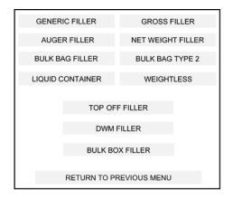
Remove power from the 5511 enclosure, then move the J12 jumper back to J11. Upon powering up the controller the selected filler type will be the only type available.
