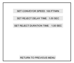
Set conveyor speed appropriate for the length of the scale and product length to allow for adequate weigh time.
