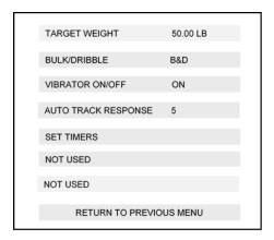
Enter the target weight, settings for bulk only or bulk & dribble, and if your equipment is equipped with a vibratory settler on the bag chair, enable (turn ON and set a value). Other recipe variables include:
