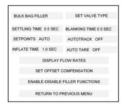
Many of the items in this screen are described in section 5.2 of this chapter. Items unique to the bulk bag filler include Inflate time and Filler Functions.
