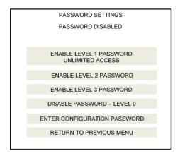
Level 1 password is the Administrative password and provides rights to enter all screens and adjust or calibrate any feature of the 5511 controller.
