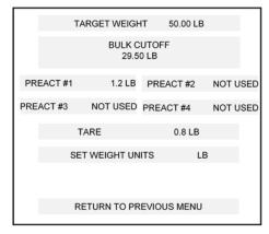
The manual set point values are purely empirical and set based upon the user's real-time experience with a fill. Set the values low and fill a bag. Once the filler's performance is known the values can be adjusted to provide the best accuracies and final fill weight consistency, verses fill time. In this mode the operator is presented with a screen showing adjustments for the Preact value.
