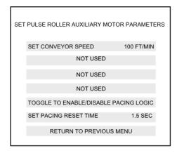
Pacing logic is enabled or disabled by touching the "Toggle to Enable/Disable Pacing Logic" button. If enabled this function relies upon the use of photo-eyes, as described in section 4.2.1, above.
