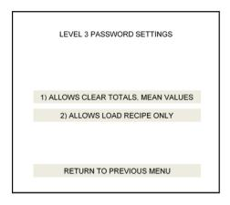
Level 3 password is typically for operators, and restricts their actions to simply loading a recipe from the main "Run" screen, or this *and* the ability to clear statistics during a run.
