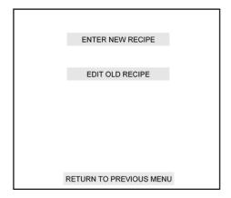
Entering a new recipe will assign the next sequential numbered recipe. You cannot select the recipe number to assign to a new recipe.
