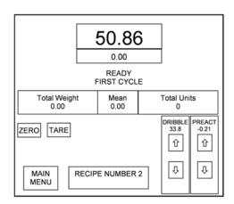
The operator can quickly tap the screen to increase/decrease values for the Dribble cutoff point (if any) and the Preact value to achieve the best possible final fill weight accuracy. The values and adjustments are tracked and updated for the recipe.
