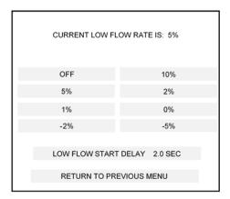
The second type of broken bag detection is within the recipe, along with target weight and several variables specific to the recipe. This broken bag detection method is based upon time alone. If the fill does not complete within the time value set in the recipe the fill will be aborted.
