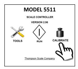
A series of screens prompt the operator through the calibration process, with the first screen offering time/date confirmation and settings to correct:
