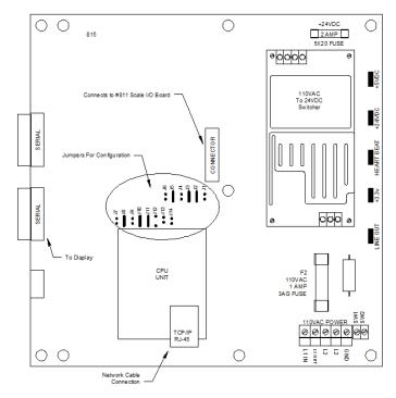
To use the 5511/6611 as a checkweigher, place jumpers as shown in this table.
