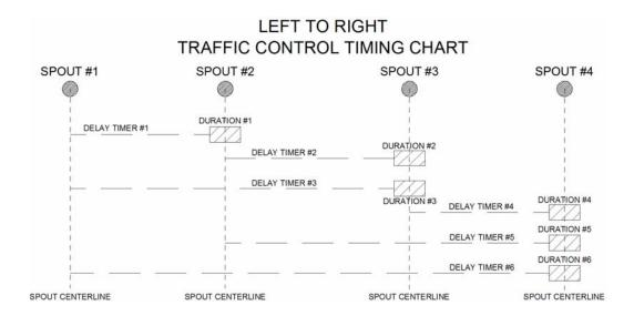
We recommend setting all timers to 2 seconds, then monitoring production and adjusting timers up or down to achieve the most efficient spacing and timing.
