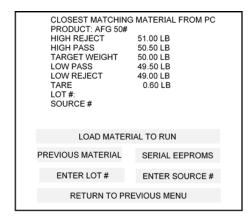
The operator begins typing the name of the recipe and the closest match will appear on screen. If it's not the correct match the operator can continue typing until the proper match appears. The operator will then select the match and the recipe parameters will be transmitted from StatPak-PC II to the controller and will load as the current recipe to run.
