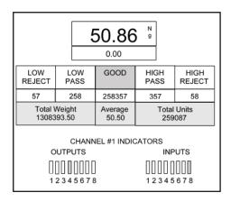
As each input is actuated; switch, photo-eye, sensor, etc. the corresponding input number will change from a white background to green. As outputs are turned on, the corresponding output number will change from white background to green. There may be more than one input and/or output on at one time.
