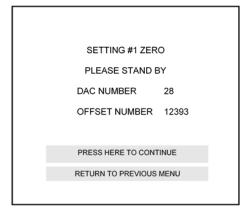
The DAC Number represents the actual Digital to Analog Conversion being executed within the 5511 controller. This value will vary from 0 to 1024 counts, and is typically in the 2 digit range. A value falling close to 0 or increasing upwards of 1024 indicates that the controller is having difficulty adjusting for the scale and deadload.
