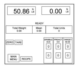
Prompts are provided for adjustment of the Target Weight, Dribble (Bulk Set Point) and Pre-Act. Double displays show live zero and the final weight of the last fill or real-time progress of the current fill.
