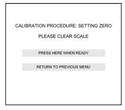
This screen prompts the user to clear the conveyor or filler, then press the Green "Press Here When Ready" button to proceed. The 5511 will run an internal potentiometer to adjust to match the scale output and establish a Zero operating point. A screen will display progress of this zero setting, showing a DAC number and Offset number:
