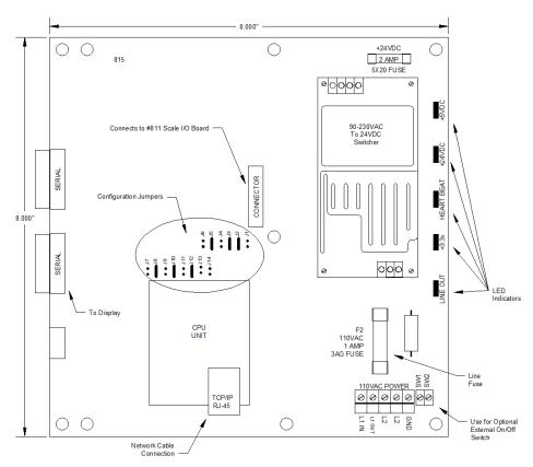
Jumper J10 should be in place to designate the controller is configured as a filler controller Jumper J11 is moved to J12 to enable configuration of a specific type of filler
