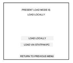
StatPak-PC II recipes are called by the operator when they press the "Recipe Number" button at the bottom of the Run screen. This sends a query to the StatPak-PC software and the following screen is displayed:
