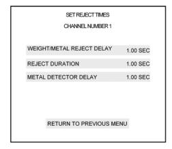
Checkweighers wired directly to the reject device will use the WEIGHT/METAL REJECT DELAY timer to set the amount of time it takes the package to reach the exit of the scale conveyor to the reject device. REJECT DURATION is the amount of time the reject device solenoid valve is actuated to drive the off-weight package from the production line.
