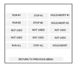
Pressing "Run" for any active scale will start the fill process. Pressing "Stop" for any active scale will bring the current fill to completion, discharge and go idle. Pressing "Hold/Abort" for any active scale will immediate stop the filling process and hold the product in the weigh bucket. If the operator presses this button again the fill will be aborted and discharged, if a bag is in place.
