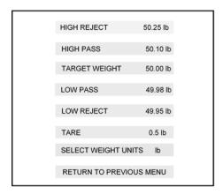
Enter the Target weight and reject limits to suite the application needs. If the checkweigher has been configured as a 3-zone scale the Low Pass and High Pass zones will not appear.
