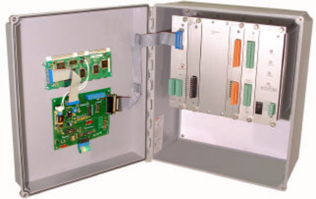
Internal View of Controller
